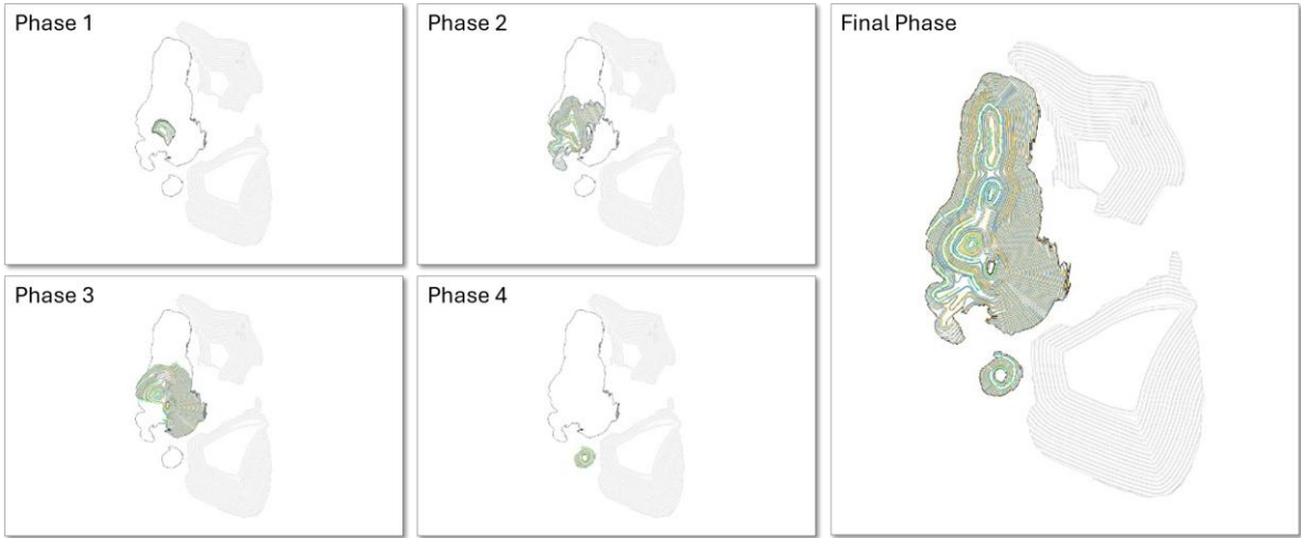
Figure 98: Taperebá Open Pit (Phase 1-4 and Final Pit) Source: Amapá Minerals — Amapá Project Technical Services, 2026
